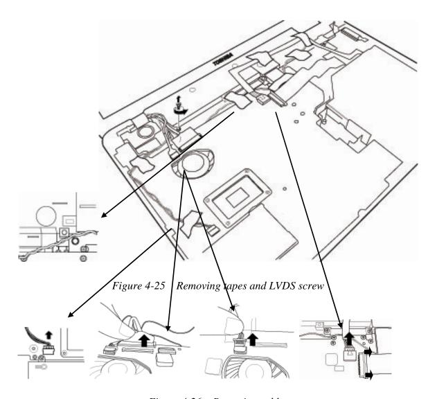
Figure 4-26 Removing cables
